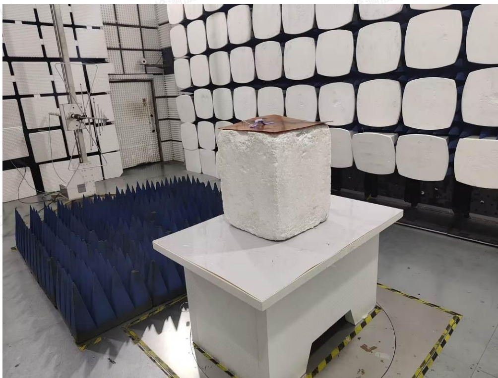
Radiated Emissions Measurement (Below 1GHz)
